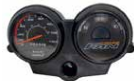
PAINEL FAN125 05-08 AUTOTEC
